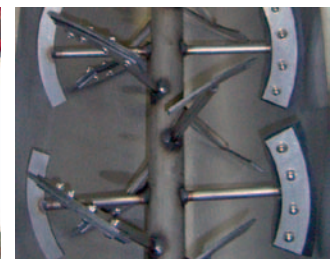
Secondary mixing unit
